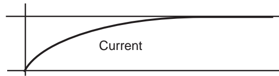
Figure 6.7-2 — Current Build-up in Phase
