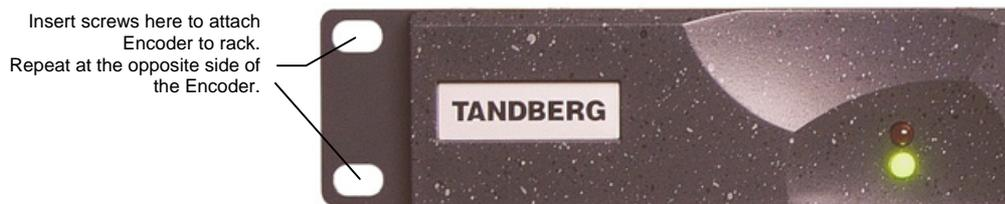
Figure 2.1: Fitting the Encoder into a Rack (1U Encoder Shown)
