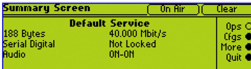
Press the Cfgs softkey for quick access to the Config menu
