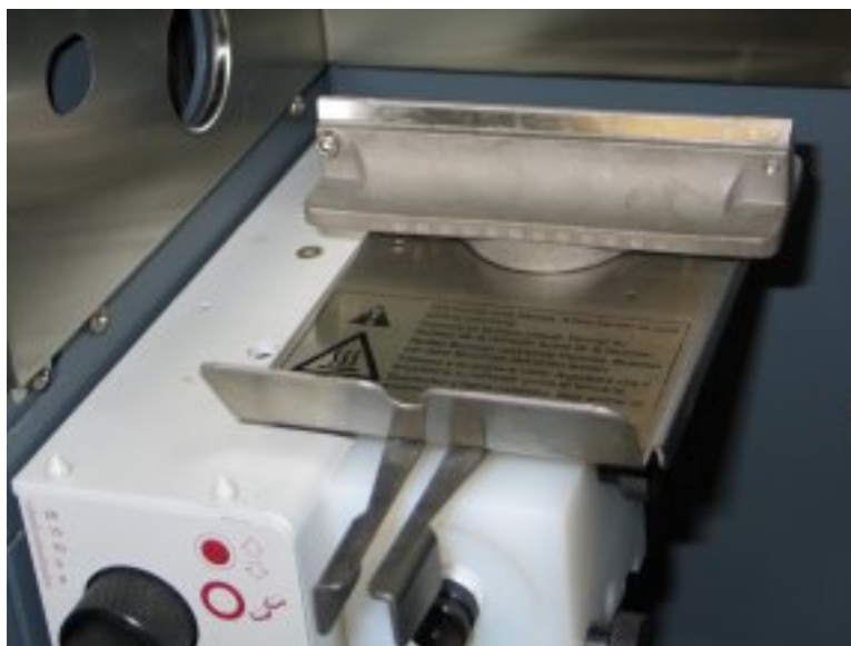
Figure 5. Mark 7 burner without holder
