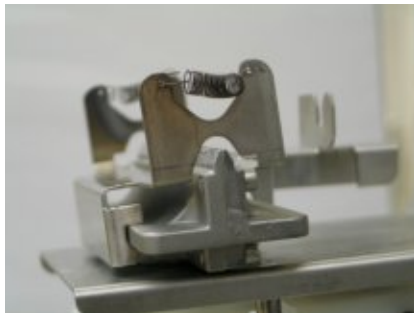
Figure 8. Lowering the cell holder into position on the Mark 7 burner
