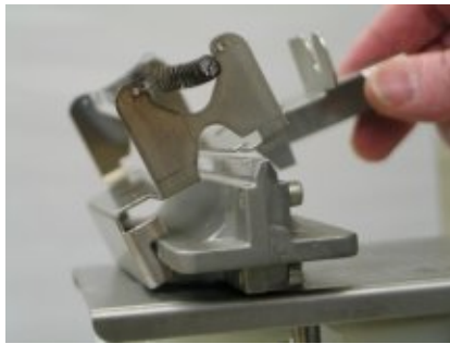
Figure 7. Cell holder pulled forward with cut-outs hooked around burner edge
