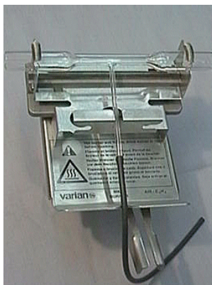
Figure 16. Mark 7 burner with standard absorption cell in cell holder positioned on top
