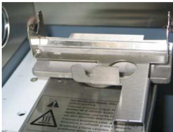
Figure 9. Mark 7 burner with holder in position
