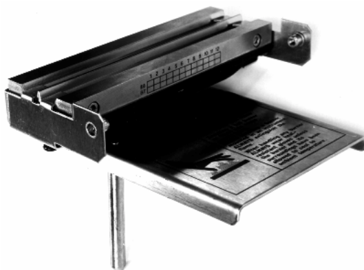
Figure 11. Mark V burner with burner clamps installed
