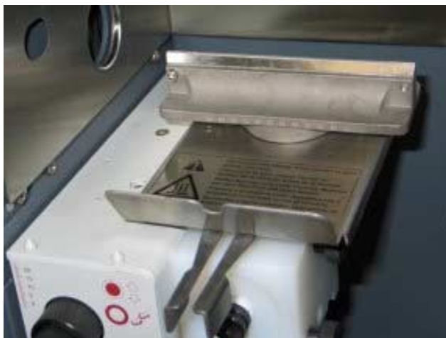
Figure 5. Mark 7 burner without holder
