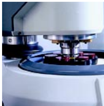
The VECTOR Power Head gives the operator the choice of preparing samples using single or central force application.
