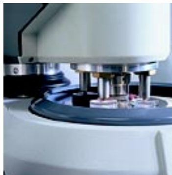
The VECTOR Power Head gives the operator the choice of preparing samples using single or central force application.
