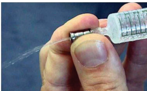
Figure 41. Cleaning the check valve
