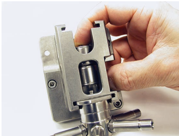
Figure 55. Installing the piston chambers
