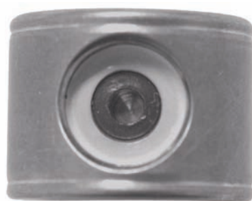
Figure 48. View showing the piston bore with a properly seated seal
