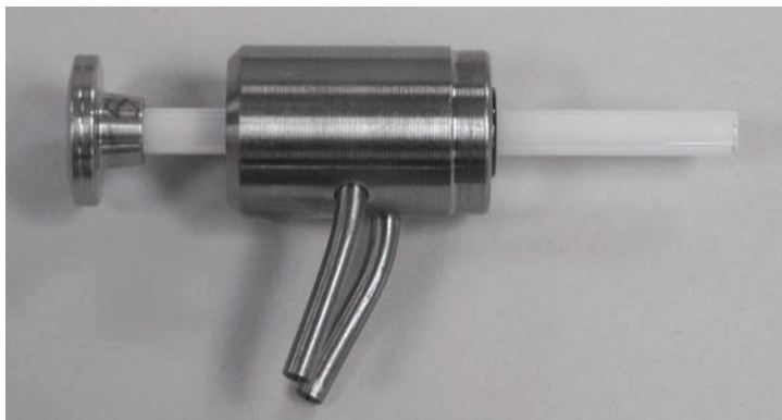
Figure 45. Seal installation tool (piston and piston guide bushing)
