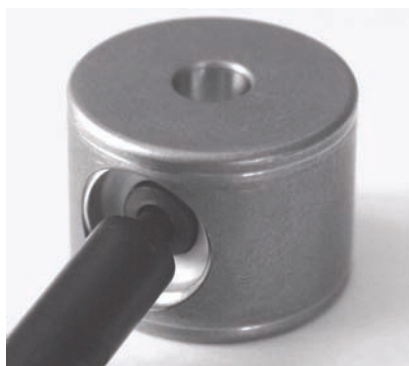
Figure 43. Removing the used primary piston seal
