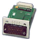
The typical use for V.35 port module are various data applications via connected router, ATM access device and the likes. Could be used with video/voice codecs, etc.
