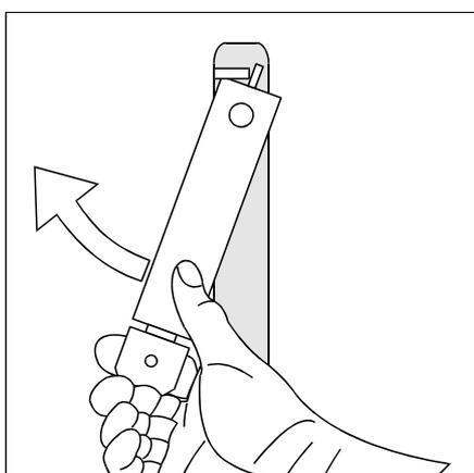
⇐ Turn the outside tracer (15) in a clockwise direction and pull it up and out.
