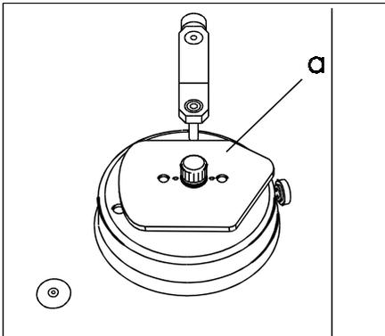
⇐ Clamp the outside tracing template (a) in position and screw tight.
