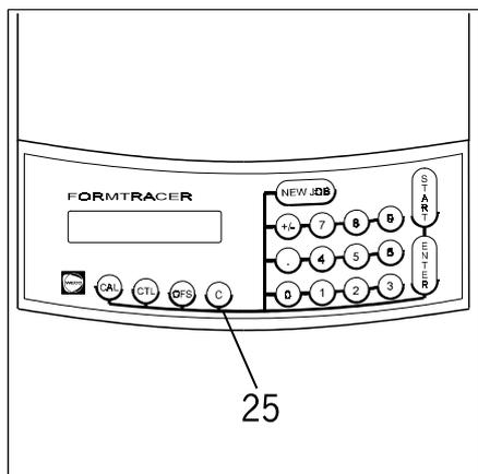
← The tracing operation can be cancelled during tracing by pressing the "C" key (25).
