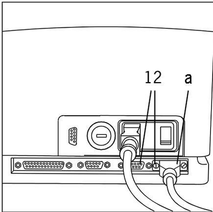
⇐ Plug the FormTracer's CL cable (b) into one of the CL ports (12) and connect to a CL port of a different CMS appliance.
