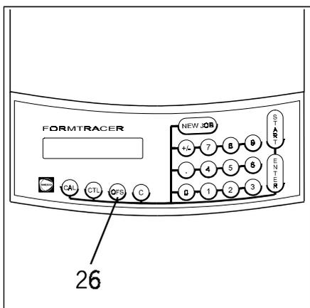
⇐ An offset of 0.3 mm for plastic frames can be entered by pressing the "OFFSET" key (26). The activated offset appears on the display.
