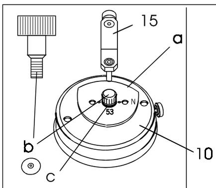
⇐ Tighten pattern (a) with screw (b).
