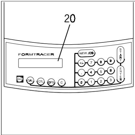
← All error and warning messages must be acknowledged with the "C" key (25).
