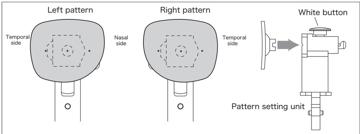
**3** Start tracing as same as Step 2 to Step 4 of “2.4.2 Pattern tracing” (Page 34). Press the Left-eye tracing button (Ⓛ) for the right eye or the Right-eye tracing button (Ⓡ) for the left eye in demo lens tracing.
