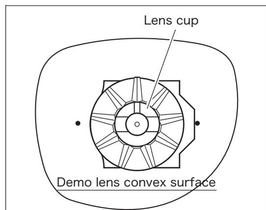
**2** Fit the lens cup into the pattern setting unit.
