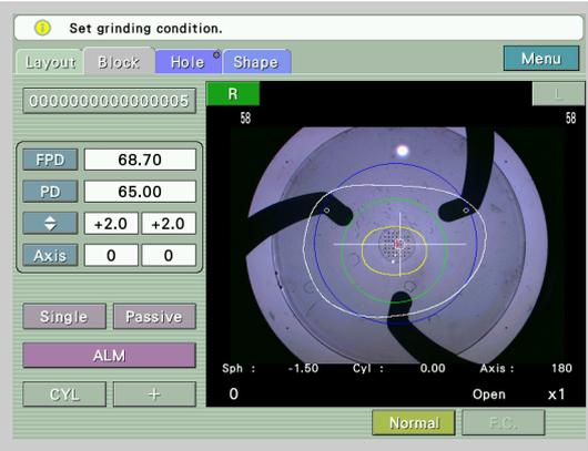
When the cup mark changes into the oblate ellipse, block the lens with a lens cup for half-eye lens.
