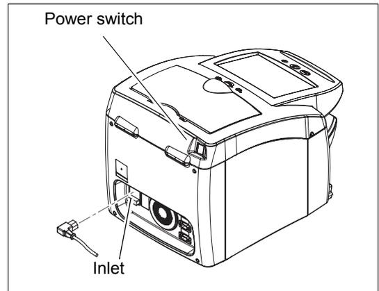
**CAUTION** The electrical outlet must have a grounding terminal.
