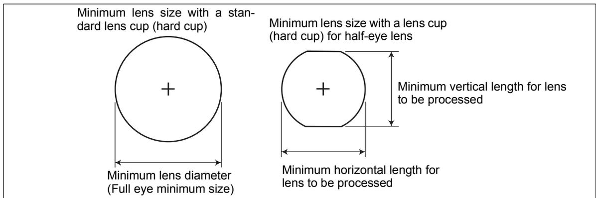
Minimum lens diameter for processing with the lens edger
