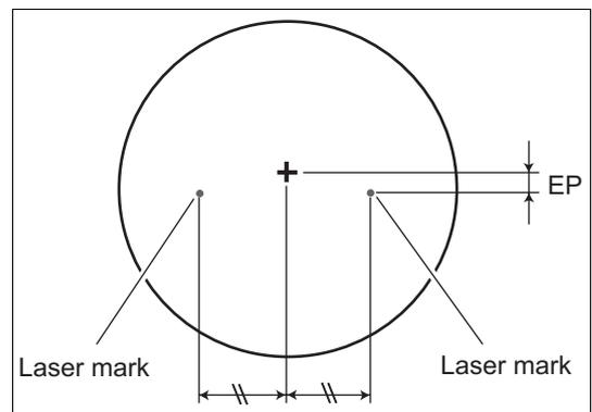
The ICE-1000 automatically detects the marked laser marks of the lens and blocks the lens.
