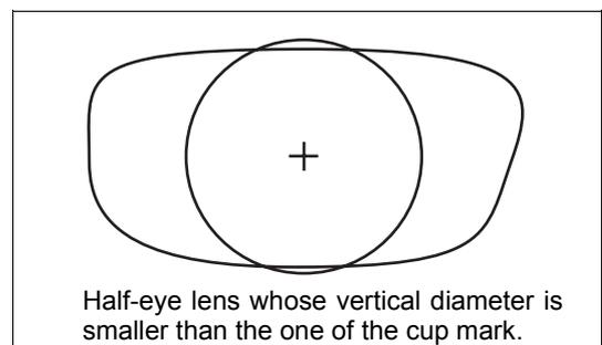
If the standard lens cup (hard cup) is continued to be used, the adapter or lens clamp may contacts the processing wheel because the distance between the blocking point and lens edge is short.
