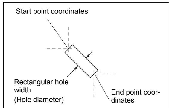
For other holes (simple hole, counterbored hole, Jewel holes 1 to 3), the hole center position is specified.
