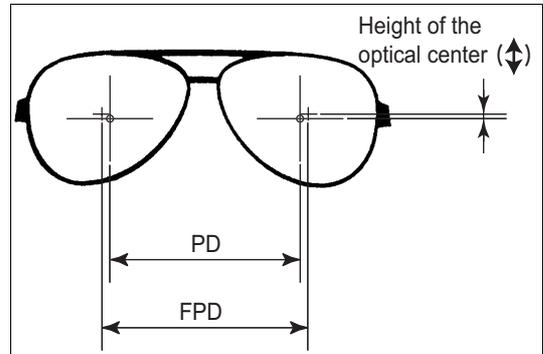
The DBL (width between the nasal ends of the left and right frames) can also be entered instead of the FPD.
