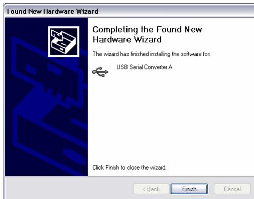
Click Finish, the Found New Hardware Wizard now starts over again because a driver for Serial Converter B needs to be installed, follow the directions above.
