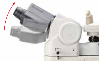
View angle is adjustable by 10° to 30°.
