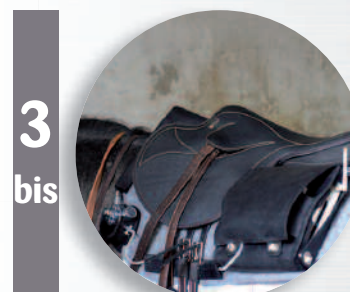
3 bis The transmitter-recorder is attached to the saddle pad
